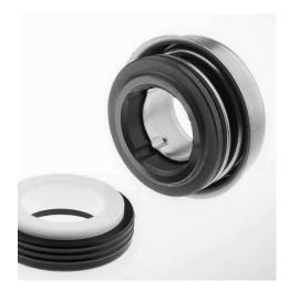
Stationary mechanical seal in inch dimensions. Spread throughout the world, this type of mechanical seal has reached an unsurpassed quality level. The BT-A2 features all carbon or high quality resin impregnated carbon, aluminium oxide 96 %, is stationary and the rubber bellows are glued on collar. Static air pressure test to 100 % production. Excellent solution for swimming pool pumps.
